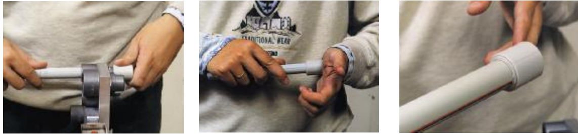
Figure 6: The heated tool socket welding – a fast and simple procedure
