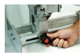
5. Insert pipe and close MTD MultiClamp. Tighten both knobs to fasten in place.
