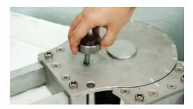
4. Adjust clamping elements toward or away from fitting as needed, and tighten slider knobs to secure them in place.
