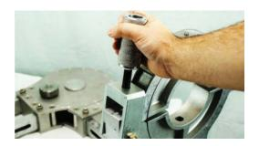
2. If needed, place appropriate size liner (4", 6", 8") into MTD MultiClamp. Tighten holding pin into hole in liner, securing liner to MTD MultiClamp.
