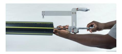
2. Expand fixation assembly into inner diameter of pipe by turning the locking expansion knob clockwise.
