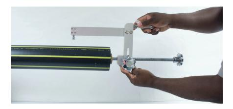
3. Set position of blade to match the requested scraping length by pushing above button and move the scraper body forward.
