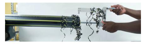
10. Loosen the pilot arm locking knob and raise pilot arm.
