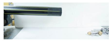
11. Loosen the expansion knob and remove both scraper and shavings from pipe/fitting.
