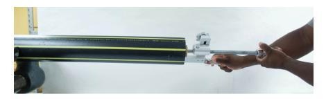
7. Hold hand grip and expansion knob during scraping to help stabilize the scrapper.
