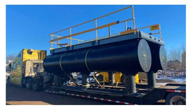
ISCO Marine can provide HDPE pipe floats for floating walkways and pump barges to create easy access for the mine and aggregate industry across North America. HDPE pipe is ideal because of its robust characteristics.
