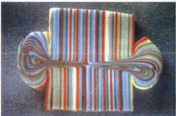
Cross section view of butt fusion melt pattern with bead
